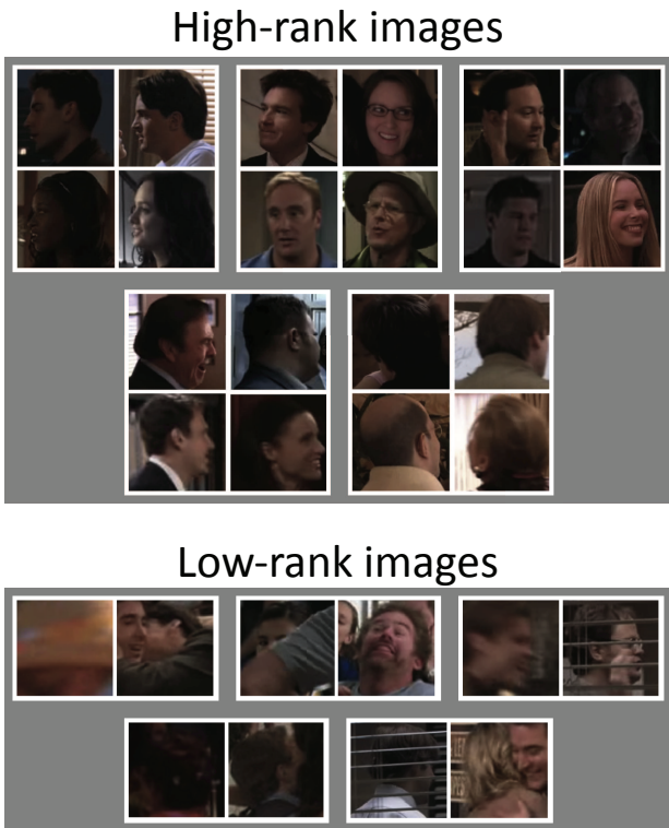
Figure 6. High/low rank images – images with highest and lowest confidence scores in each cluster. High-rank images correspond to five discrete head orientations. Low-rank images are due to: i) the regression procedure fails to localize the head region; ii) subject exhibits a rare head pose; iii) the head is occluded; or iv) the image patch has low resolution, low contrast, or motion blur.
