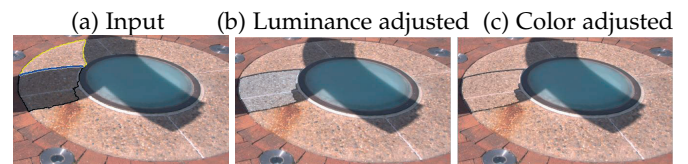
Fig. 2: Shadow region relighting using lit neighbor. (a) Shadow region and lit neighbor: shadow region depicted with black boundaries, lit neighboring region depicted with yellow boundaries, common boundary drawn in blue. (b) RGB reconstruction showing the result of histogram matching on L channel for the shadow region. (c) Shadow region relit, results after the adjustments in a and b channels.
