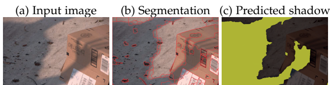
Fig. 11: Failure due to segmentation. Soft and elongated shadow regions, such as the shadows created by the fingers, are hard to detect, partly due to the error during superpixel segmentation and grouping. This process may produce regions that contain both shadow and non-shadow pixels.
