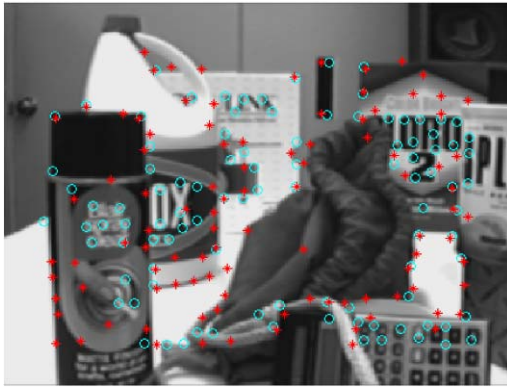
Fig. 8 (Color online) Selected feature points based on two different criteria. Cyan circles: 100 points selected using Shi & Tomasi's criterion. Red stars: 100 points selected using our criterion. Selected feature points of each method are at least 10 pixels apart
