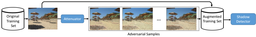
Fig. 1: Adversarial shadow attenuation. The attenuator takes an original shadow image and generates different adversarial shadow samples to train the shadow detector.
